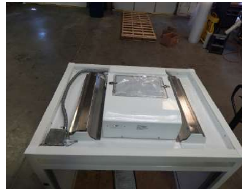
Filter Unit top view, with filter installed
